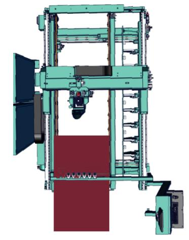
2. The door is positioned against the stop and the door is clamped.
