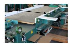
These buttons adjust the door width into the machine. The reference of the starting point varies upon the way the machine fence is aligned to incoming machinery.
