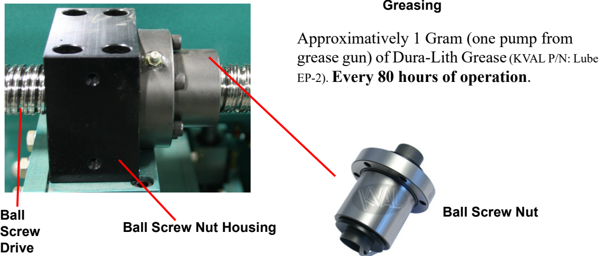
FIGURE 3-8. Example of a Typical Ball Nut
