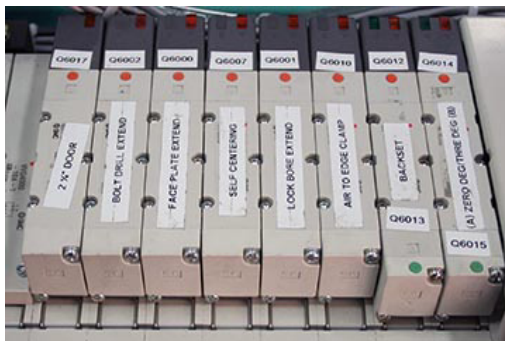
FIGURE 4-9. Solenoids in Manifold
