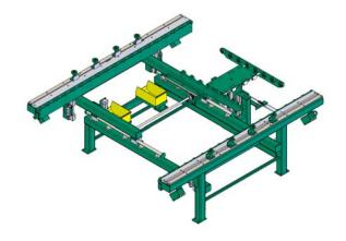
The standard Entrada-1 will accommodate doors 6'-8" high and doors that vary in width from 2'6" to 3'0". With the 8'0" door capacity option, the RKG-1 can be set up to accommodate doors that vary in height from 6'8" to 8'0". The RKG-1 will accommodate all jamb widths.
